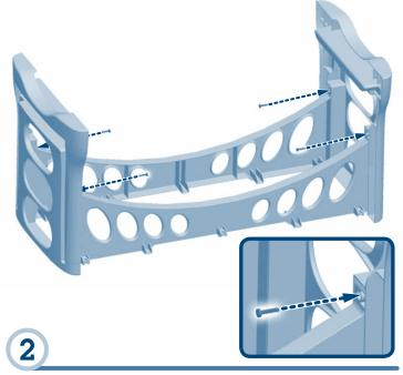
•Insert two screws into each leg support and tighten.
